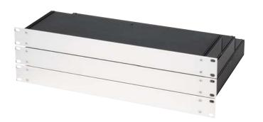
Micro 19 series is ready for rack mounting. The front panel is 3 mm thick and completely flat for easy machining and silk screening. Micro 19 series has been developed for micro-computers, modems, communications and computer peripheral equipment. Grooves in the side extrusions make mounting of PC-cards and cover plate a simple slide-in operation. Micro 19 series enclosures are available in 3 standard sizes and delivered complete and ready for assembly.
